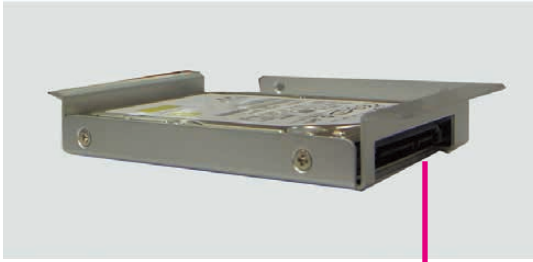
Connector side of the SATA drive
