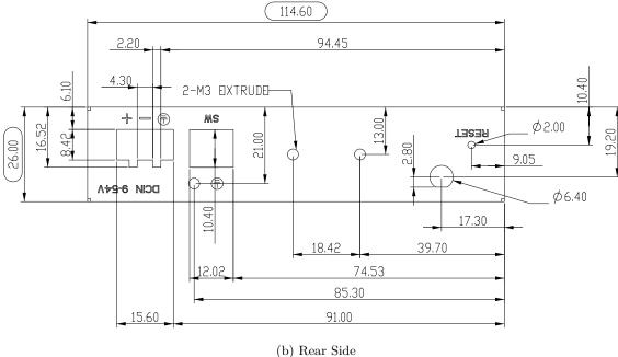
Figure 3: Mounting Positions Baltos iR 2110
